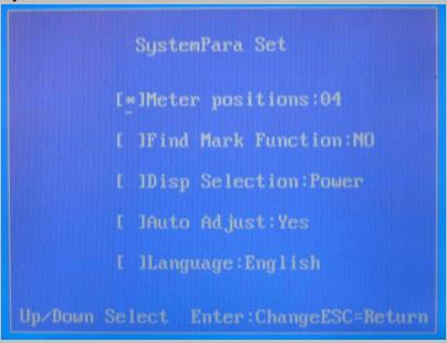
**Meter positions**: meter positions of the test equipment.
